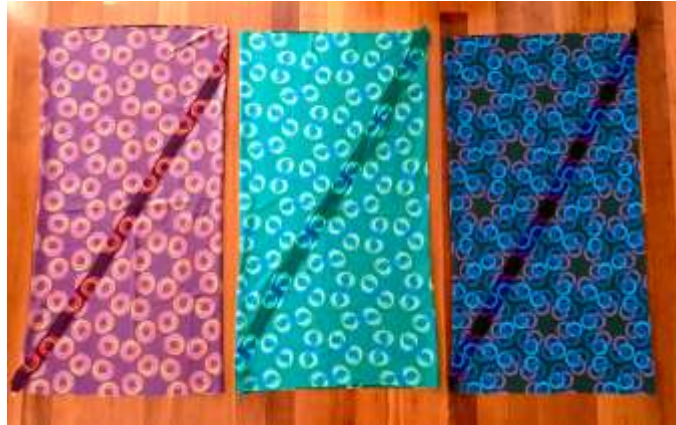
Figure 23. Sewing together the first pair of rhombus edges results in a “cylinder” with a diagonal seam. Each diagonal seam has a 4-inch opening in the middle.
