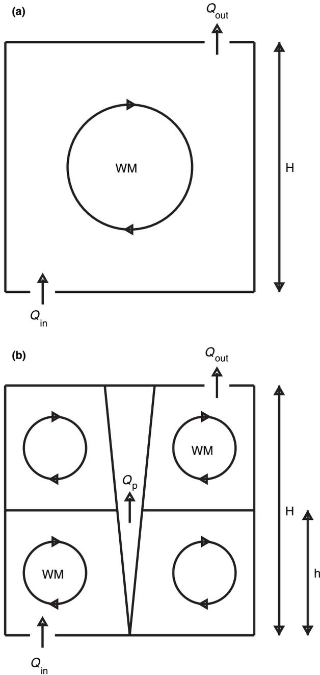
**Fig. 1** Models of displacement-ventilation systems. (a) single well mixed layer, (b) two-layer system
