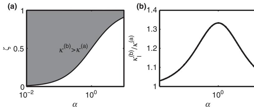
**Fig. 3** (a) Comparison of the steady state average concentration across the entire height of the space for the single layer vs. two layer models (b) Ratio of the steady state concentrations of the lower layer in the two layer models to the single layer concentration ( $\kappa^{(b)}/\kappa^{(a)} > 1$ )
