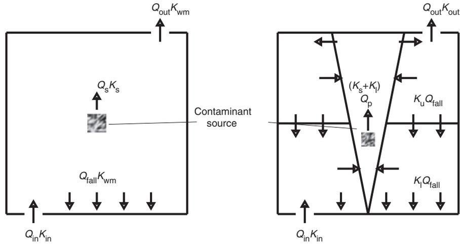
Fig. 2 A schematic illustrating the contaminant transport processes taking place in the well mixed and two-layer cases
