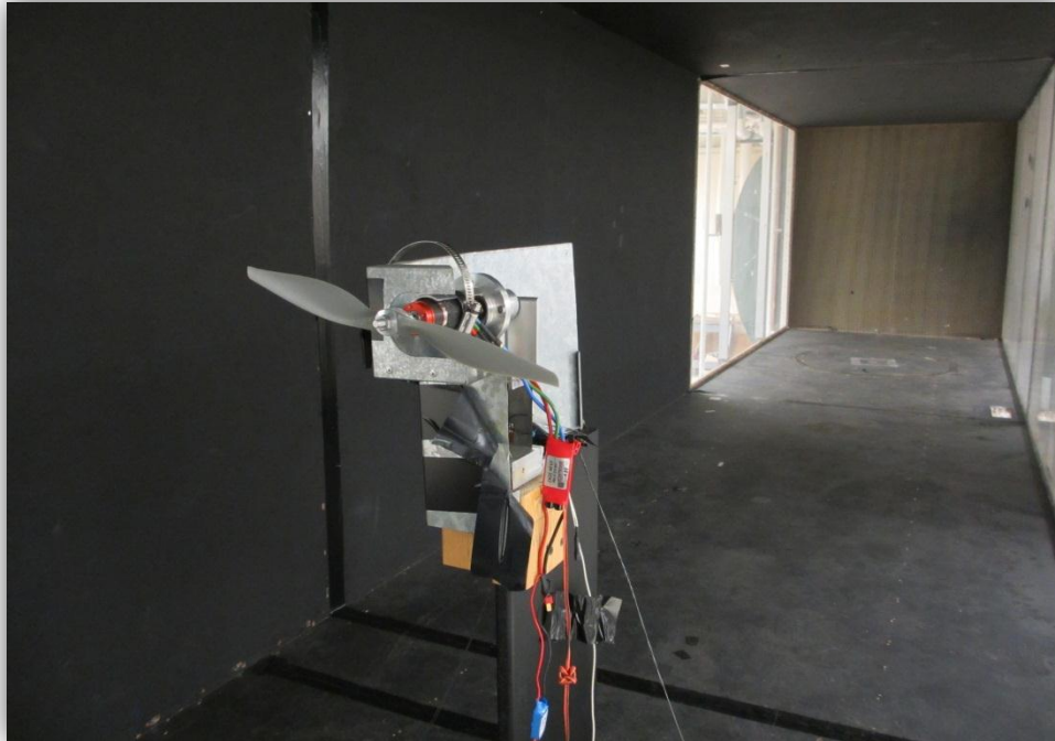
Figure 8.3 – Propulsion Experimental Test Set-Up
